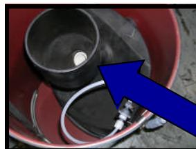
Assure sink drain fits into Purifier intake flange.
