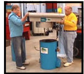
Lift over Gatorizer and assure pump is not obstructed by Purifier.
