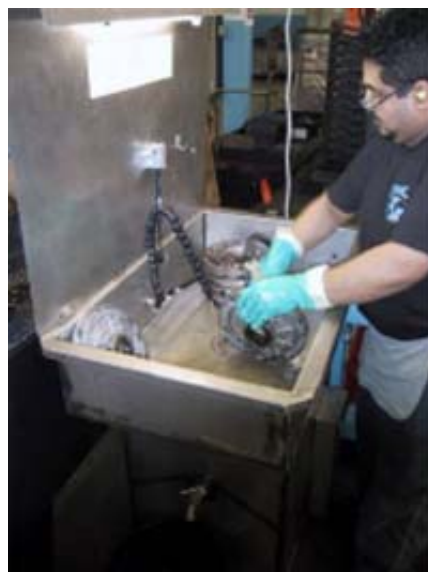
As shown above, the Grease Gator has a parts washing sink for the user
