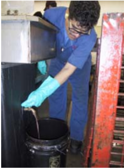
Purging oil from the collection chamber
