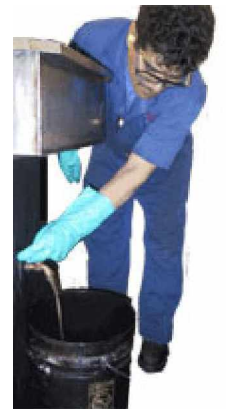
Purging the used oil from the reservoir.
